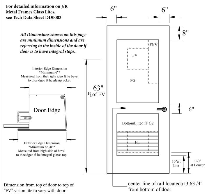
"FV" vision lite to vary with door height; minimum top rail to be 8". Dimension from bottom of door to center line of "FV" lite to remain constant at 63".
