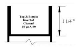
Door Standard Prep 7 gauge Hinge reinforcement 161 or .134 v blank prep Air Dry high performance gray primer
