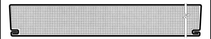
Polystyrene Insulated Core Doors Polystyrene Insulated Core Doors are available in standard 18 ga A-40 steel.
