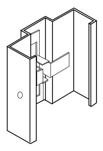
**Drywall Pressure Anchor with Dimple**
