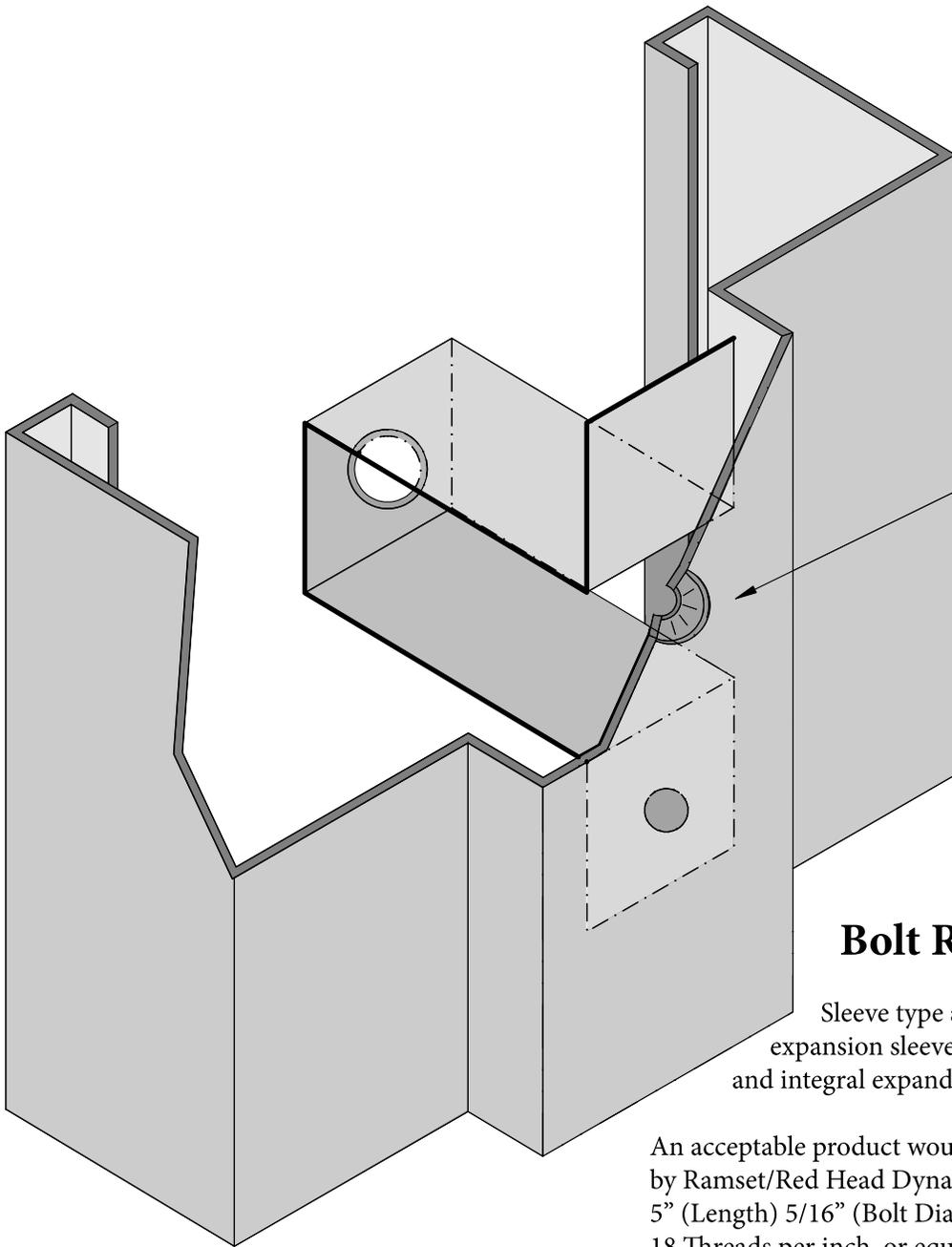
Frame countersunk to receive flat head masonry expansion bolt.
