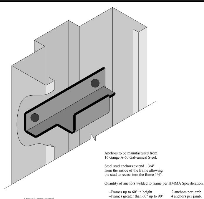
Drywall must extend a minimum of 1/2" on fire rated frames per ANSI A250.11
