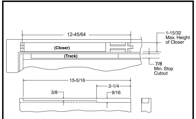
Concealed Closures are prepped either in Doors, or Frames depending upon template provided by hardware closure manufacturer.
