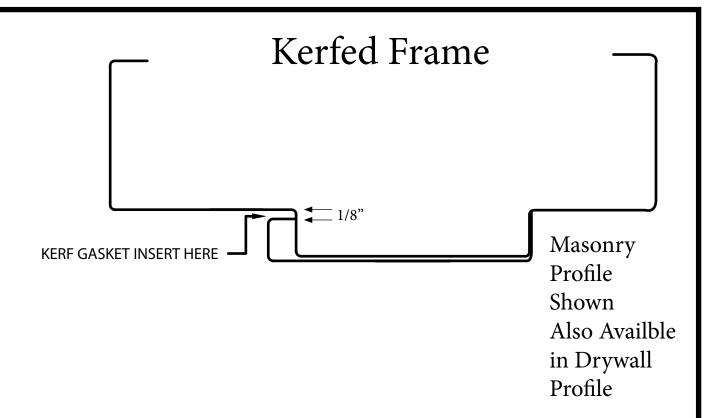
Frame gap is 1/8"wide to receive kerf weatherstrip
