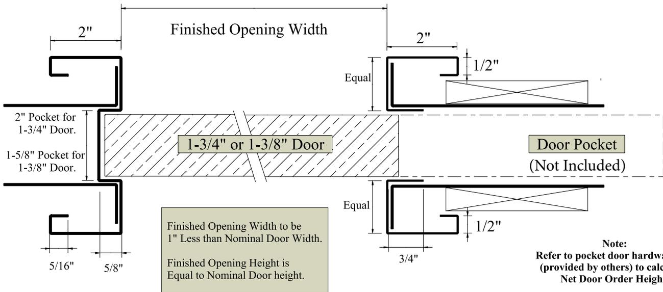
Smallest jamb depth available for a pocket door frame is 4 1/2" (3 1/2" Wall Dimension).
