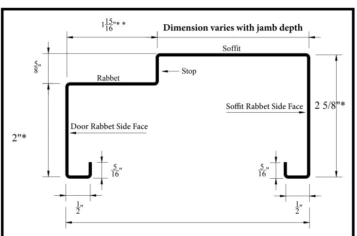
Smallest jamb depth available for a single rabbet frame is 3 1/4" (2 1/4" Wall Dimension).
