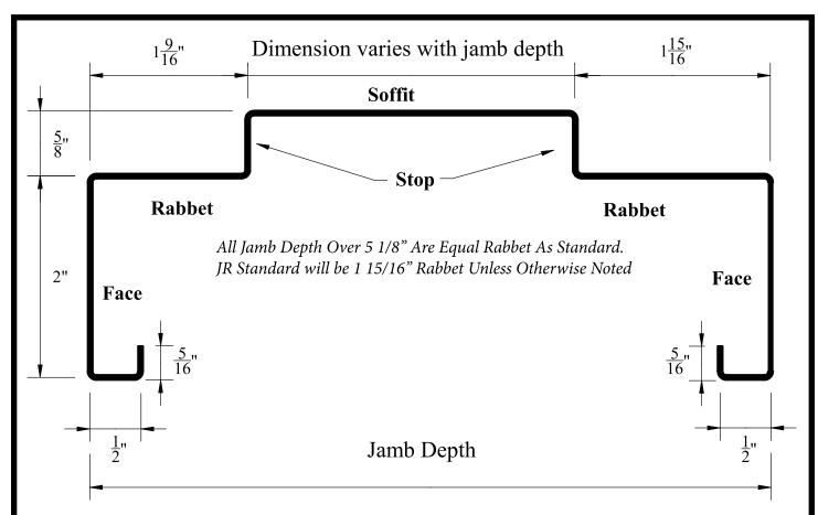
Smallest jamb depth available for an unequal rabbet frame is 4 3/8" (3 3/8" Wall Dimension). Smaller jamb depths must be single rabbet.
