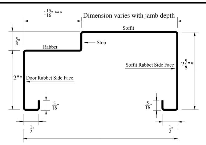
Smallest jamb depth available for a welded single rabbet frame is 3 1/4" (2 1/4" Wall Dimension).
