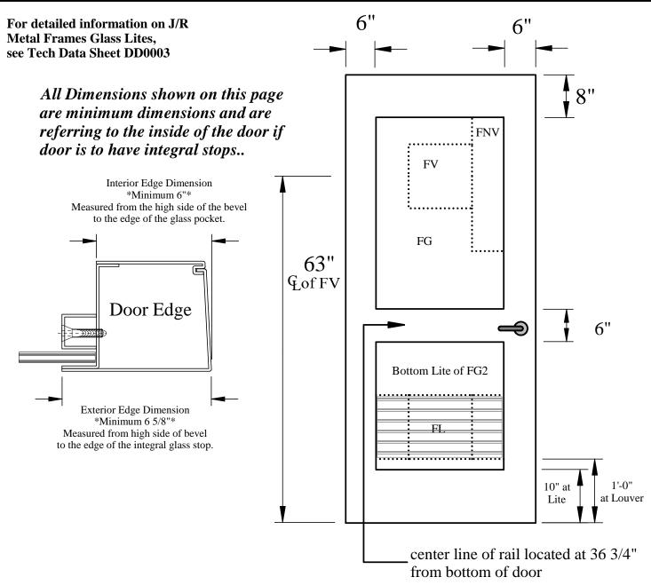
Dimension from top of door to top of "FV" vision lite to vary with door height; minimum top rail to be 8". Dimension from bottom of door to center line of "FV" lite to remain constant at 63".
